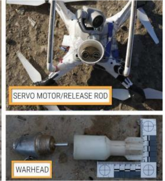
Source: Commercial Drone Modified for Projectile Drop Capability by Islamic State Operatives, Combating Terrorism Center at West Point, The Islamic State and Drones, 2018, https://ctc.usma.edu/wp-content/uploads/2018/07/Islamic-State-and-Drones-Release-Version.pdf
